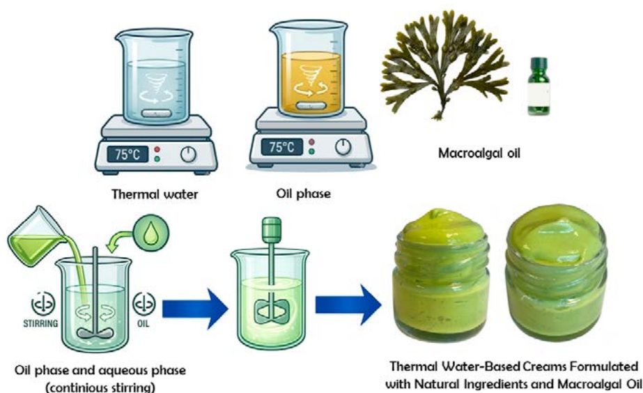
Figure 1: Schematic of the Cream Formulation Containing Thermal Water and Macroalgal Oil.
